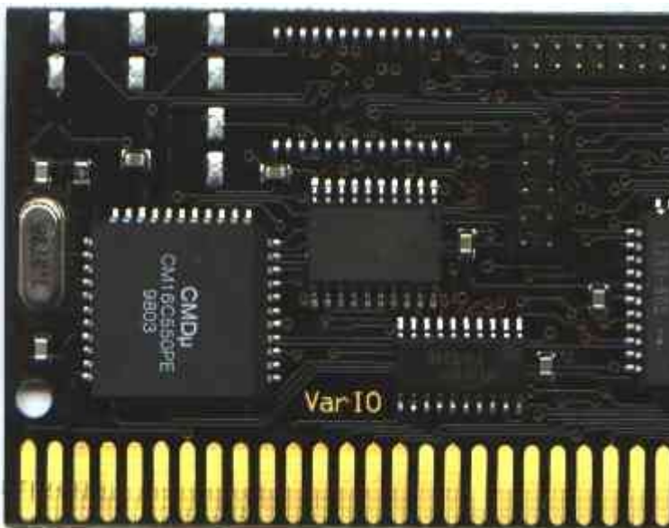
level-converter of the VarIO for Zorro/26-pin usage
