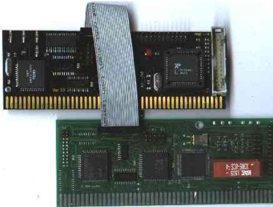
connecting a VarIO to the clockport of an ISDN-Surfer
