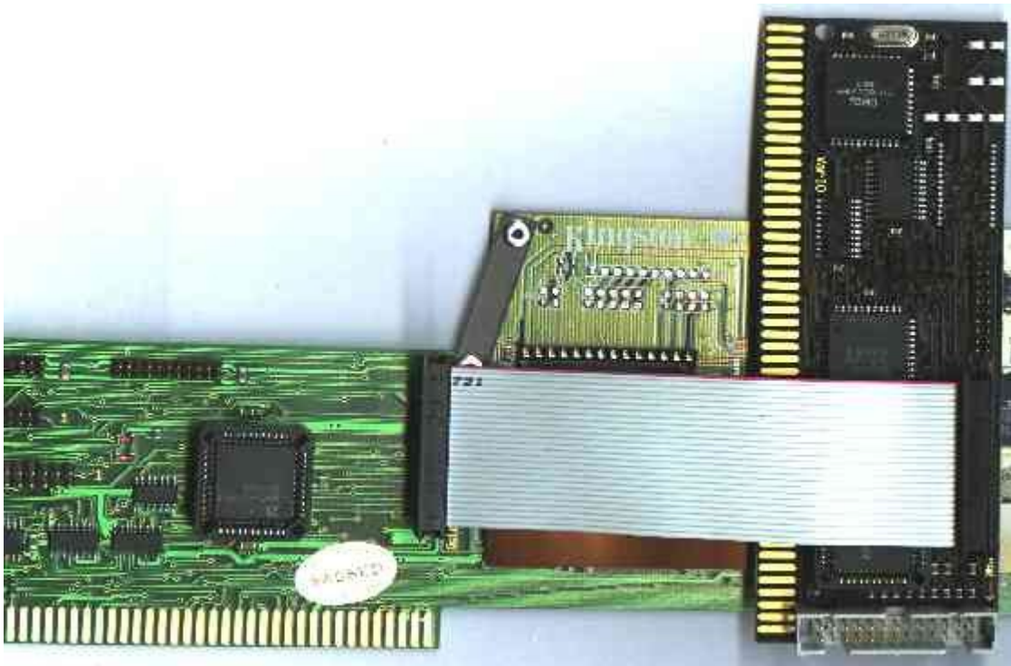
connecting a VarIO on a X-Surf ethernet board
